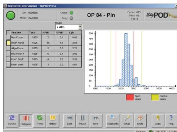
A SigPOD™ Press screen showing how the auto-learn Histogram feature reveals the distribution of insertion force failures. Specified limits can be adjusted by the user and the resulting distribution of failures is displayed prior to deployment of the new limits on the factory floor.
